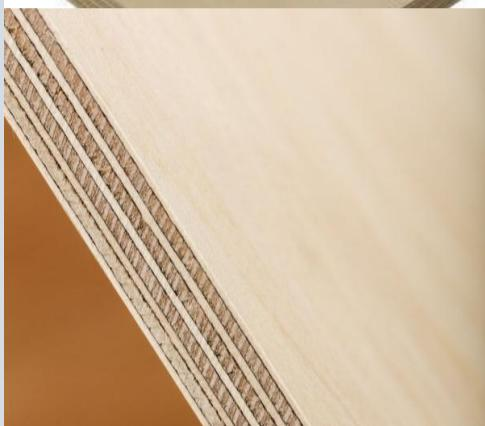
Ply or pine are great candidates to make the structure of the table from this is due to their strength and water resistance, especially if you buy marine grade or structural grade.
