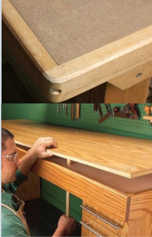
The MDF tabletop fits into a notch created by the side pieces allowing for a snug fit, and a hole at the underside for when the MDF needs to be replaced when damaged.
